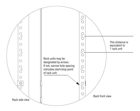
The following figure indicates proper locations for sheet metal nut locations. To ensure a level installation, the same eight rack unit locations are used on each vertical rack piece.
