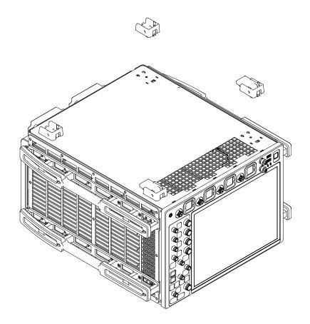
2 Remove all four feet by pressing firmly on the tab and lifting the foot off.
