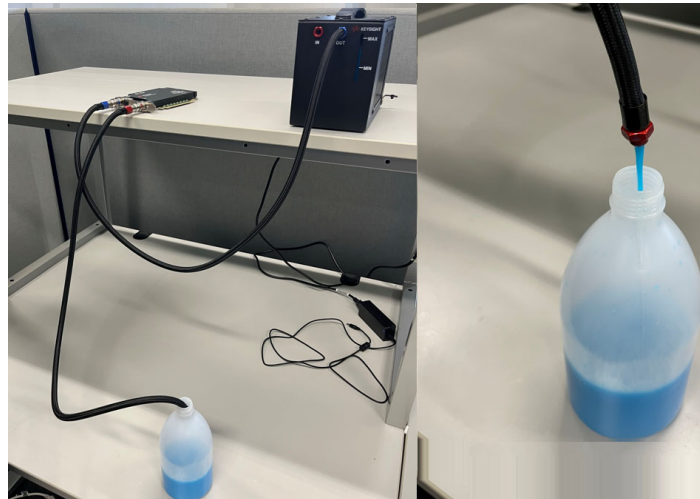
Figure 14 Emptying coolant from the Exerciser/Analyzer and heat exchanger
