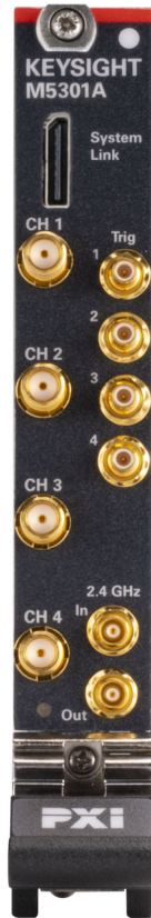
Figure 1 Front view of an M5301A PXIe Baseband AWG module
