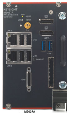
Figure 6 Front panel view of M9037A Embedded Controller
