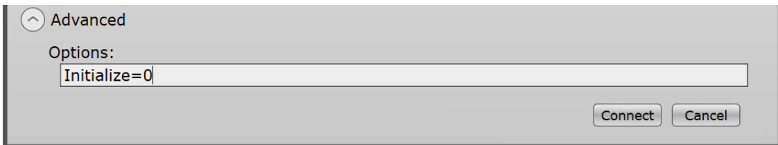
Figure 42 Setting option 'Initialize=0' to perform firmware update through SFP
