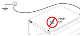
Figure 6 Establishing earth ground to the chassis
