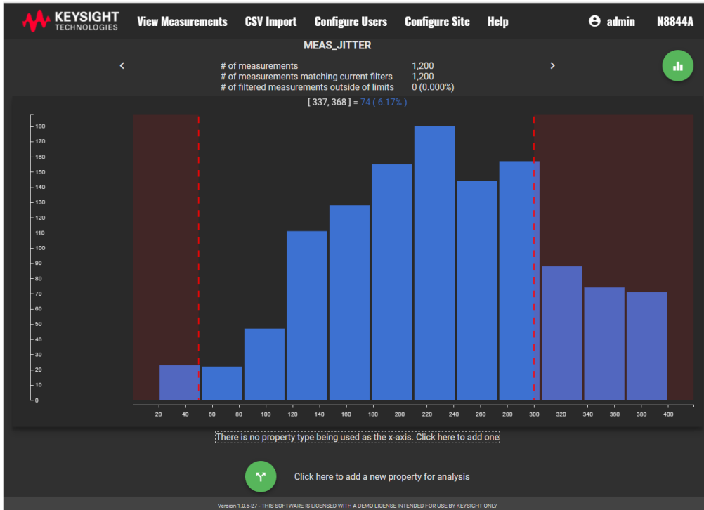
Figure 3. N8844A Visualization Tool reveals the plot of a DDR4 clock jitter measurement in histogram mode. The red zones show the upper and lower test limits of the measurement as specified in the JEDEC specification.
