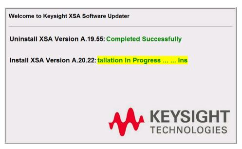
The new instrument software is being installed. The "Installation in Progress" text will roll across the screen indicating software activity. There will be several windows appearing and disappearing during this time. No interaction with the instrument is required. Please be patient the total software installation process can take 20 to 35 minutes. It will display "The software
