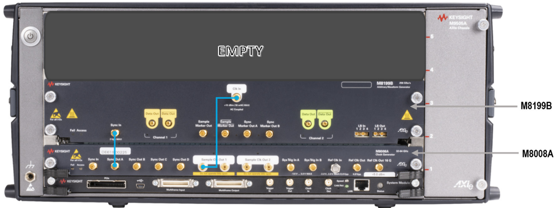
Figure 20 Connecting M8008A clock generator to one M8199B AWG module
