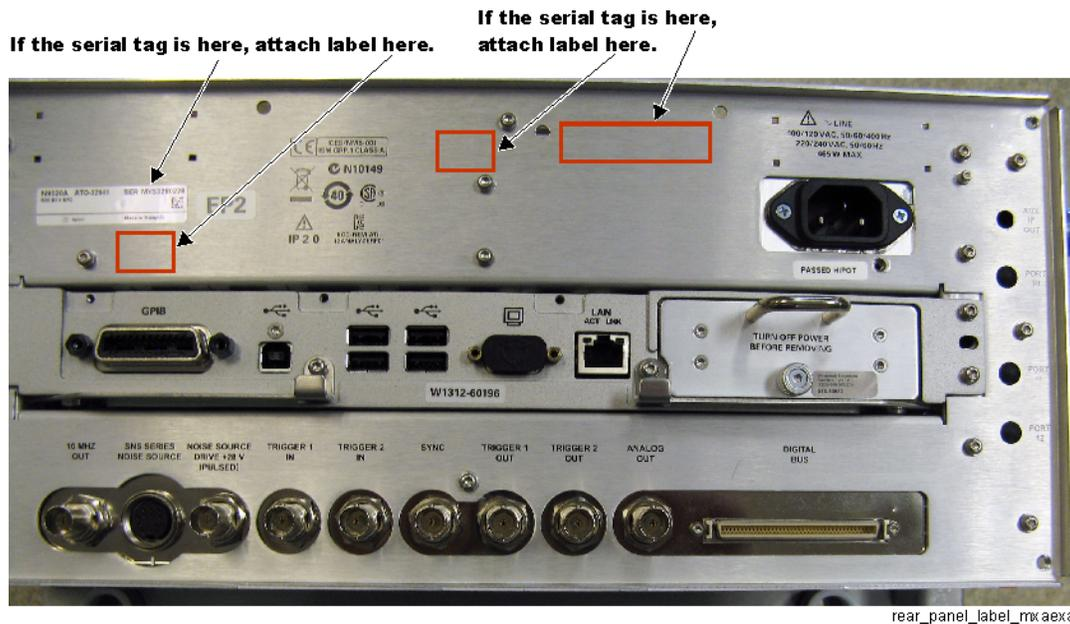
2. Locate the correct nameplate label that indicates the new frequency range of the analyzer.
