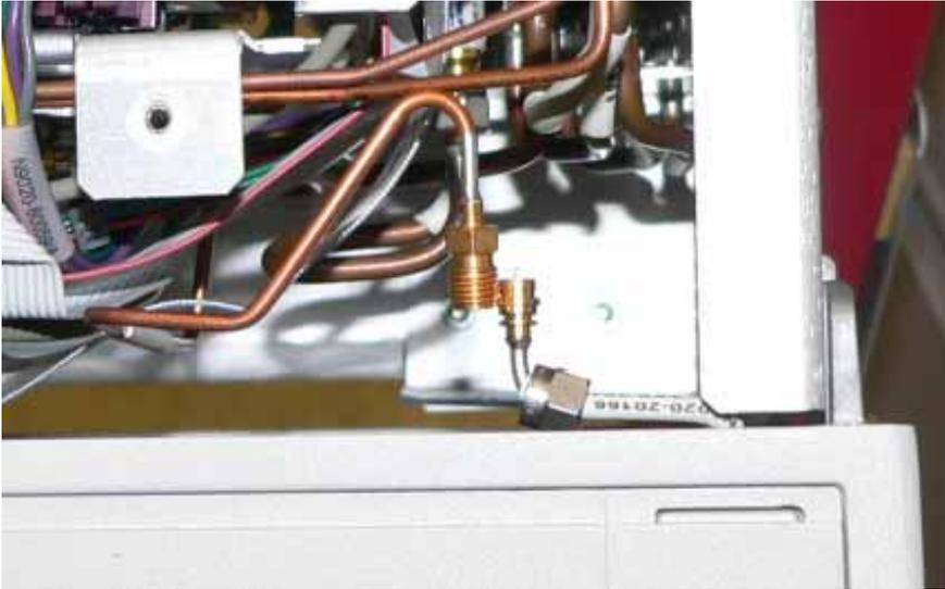
**Figure 25** W27 and W28 Properly Aligned
