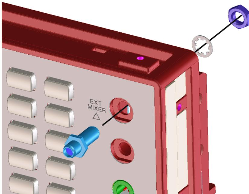
4. Locate the External Mixing, Front Panel semi-rigid coax assembly in the kit, part number N9020-20166. This is W27. Note that this cable is symmetrical; either end can be connected to the front-panel connector.
