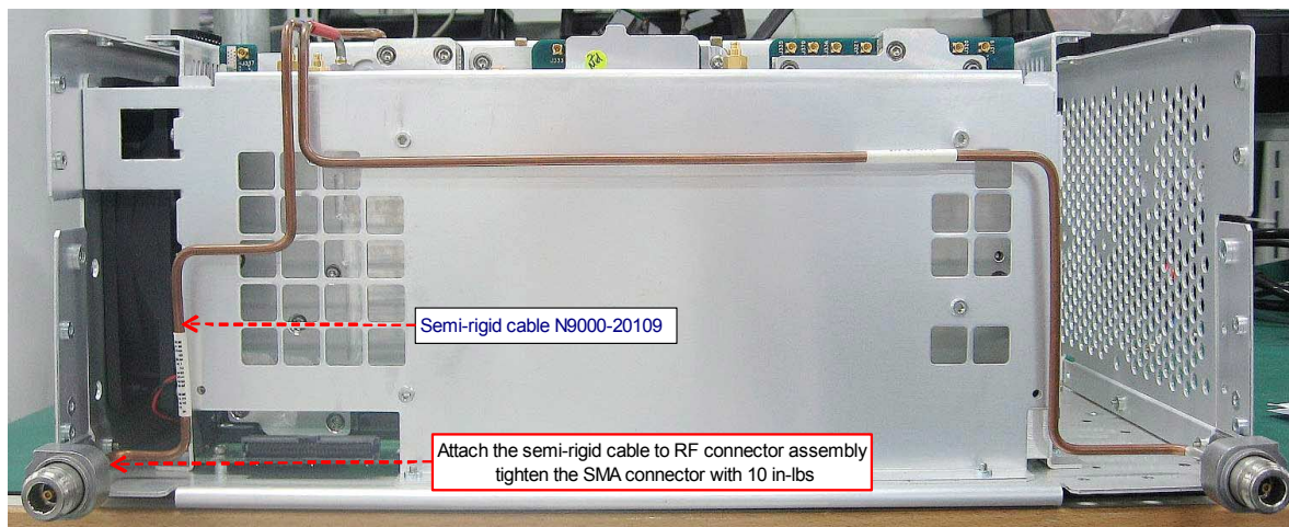
Figure 7 Install the RF Semi-rigid Cable
