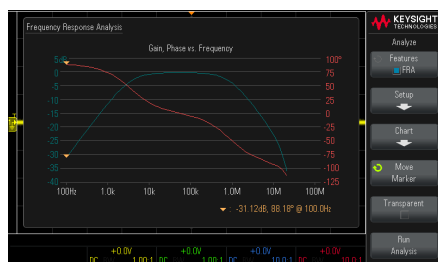
Bode plot feature for frequency response analysis
