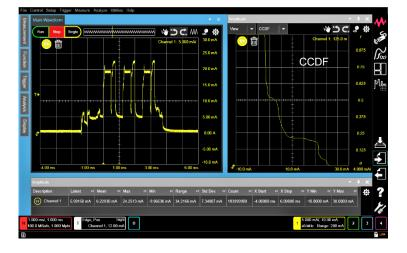
CX3300 features statistical analyses such as complementary cumulative distribution function (CCDF) or histogram on the mainframe. As a result, you can now focus on your measurement without transferring the data to your PC.
