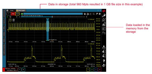
Figure 19. CX3300 can read and playback from the storage for deep analysis similar to the scope mode
