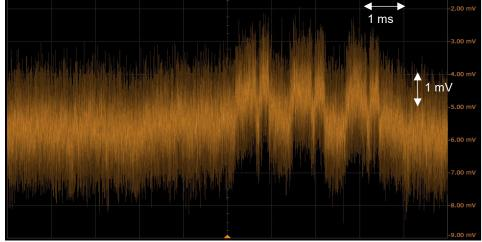
Figure 4. CX3300 captures very small differential voltage beyond a conventional differential probe
