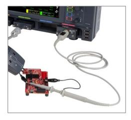
Figure 14. CX1151A passive probe interface adapter
