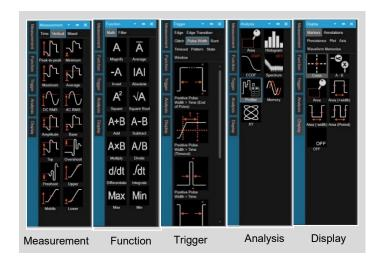
The CX3300 provides easy access to the built-in capabilities such as measurement, function, trigger, analysis, and display.
