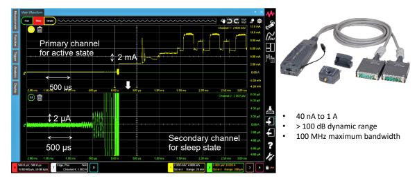
Figure 10. CX1102A measurement example
