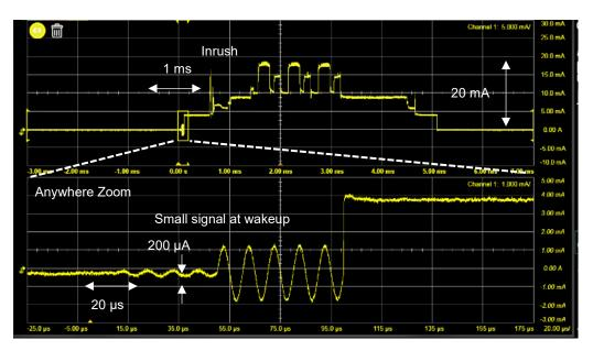
Figure 3. Precise dynamic current waveform provides valuable information to validate and optimize the circuit design.
