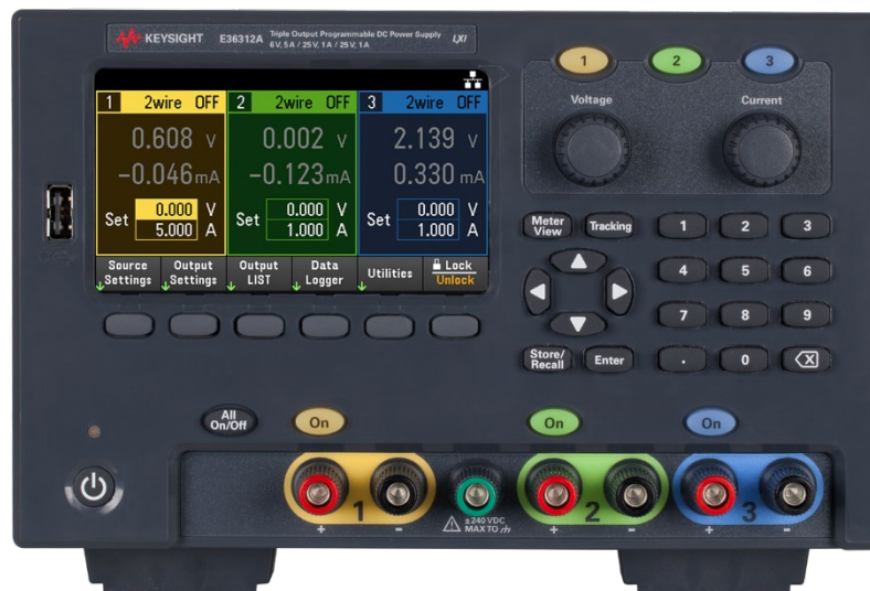
Figure A.03. The E36300 series of triple output DC power supplies.
